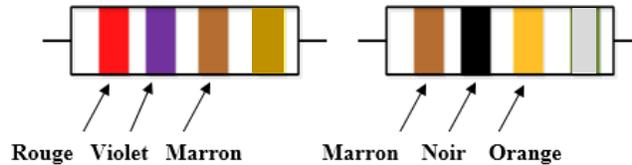
❖ **Réponse :**  $R_1 = 270 \Omega$        $R_2 = 10000 \Omega = 10 \text{ K}\Omega$
